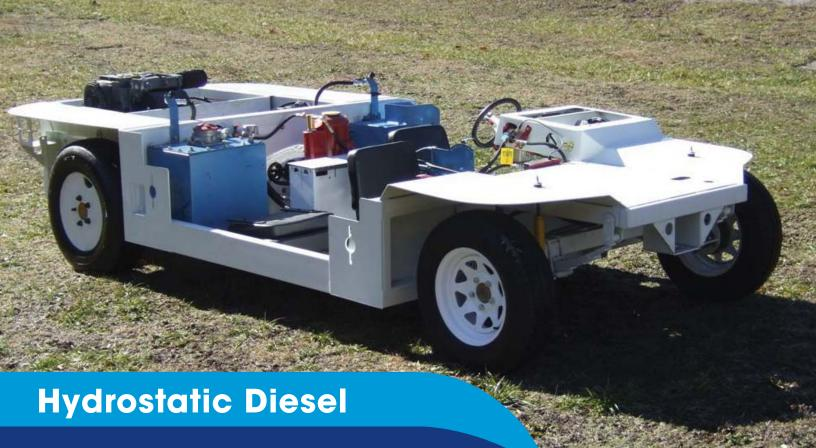
The Hydrostatic Diesel from Johnson Industries is a nonpermissible, MSHA approved personnel carrier and tow vehicle for use in underground and above ground mining. For sustained run time and pulling power, a diesel transporter is the way to go.
